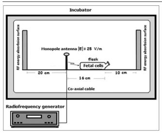
Figure 1: During the study, a GSM signal generator was used to generate radiofrequency electromagnetic radiation (RF-EMR). The RF field was set to 25 V/m. The RF-EMR exposure system applied 900 MHz RF to fetal cells
